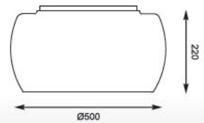
RAIN Ceiling C0076-06X-F4K9 6*G9 MAX 42W metal chrome / smoky glass / crystal drops inside IP20
